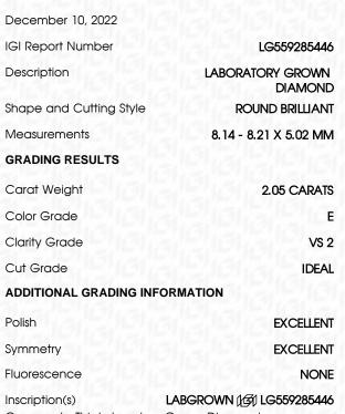
Comments: This Laboratory Grown Diamond was created by Chemical Vapor Deposition (CVD) growth process and may include post-growth treatment. Type IIa
